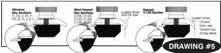
3. C124 and C135 have tiny grooves. Be sure jaw engages into a groove.
