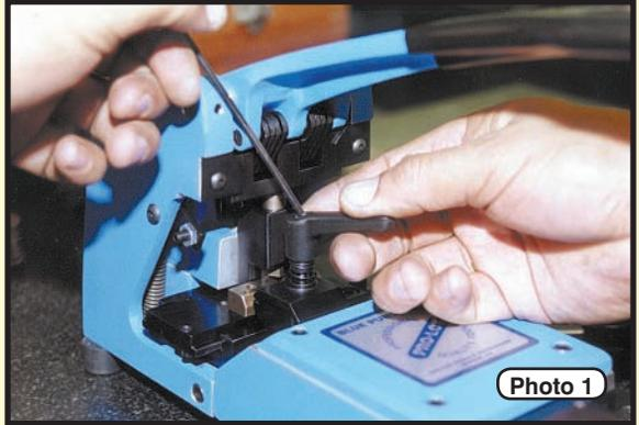
2. Loosen the top right screw on the top plate. See photo #2.
