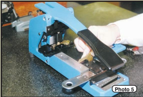
10. Re-insert the code bar to the depth cut #5. See photo #5.
