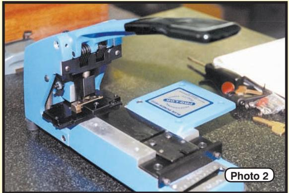
5. Tighten the top right screw in the top plate to keep the top plate stationary while you work. See photo #2.
